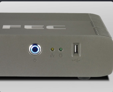
Power button, internet connection indicator, hard disk indicator and USB port is located in the front face for quick maintenance.
